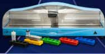
**FASTH 21** for a variety of applications listed here: Its main application is the fully automated homogenization for residues analysis sample preparation. It can be also used for many other sample preparations:
