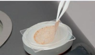
Add 10 drops from "C" bottle on membrane filter in the dish and wait until the filter is completely dry.
