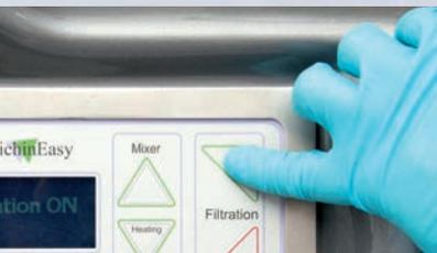
After few minutes press the "Filtration" button start. When all the washing solution has been pumped out press the "release" button 3 seconds. Remove the Filtration cylinder and wash it with clean water.
