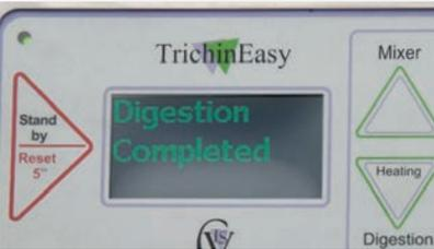
After 30 minutes (best digestion time), the instrument warns the end of digestion by a beeper and the message "Digestion Completed" will appear on display.
