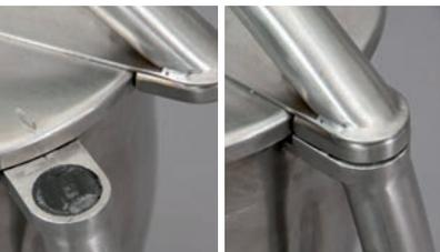
Close the Mixer and Digestion container cover turning it clockwise.
