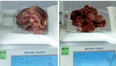
Weigh the sample and put it in the Mixer and Digestion container in quantity not exceeding 100 g.
