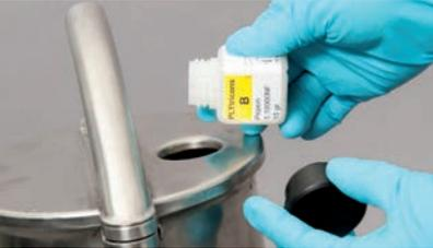
Add the content of "B" bottle (Pepsin 1:10000 NF) through the hole on the Mixer and Digestion cover. The digestion phase starts and the instrument will provide to shake and maintain the digestion liquid temperature until the digestion is completed.
