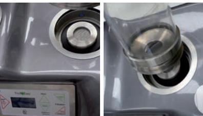
Insert the filtration holder with membrane E in the hole (right side of the instrument) then add the cylinder on top of the filter.
