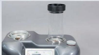
Decant the digestion liquid from the Mixer and Digestion container into the Filtration cylinder.
