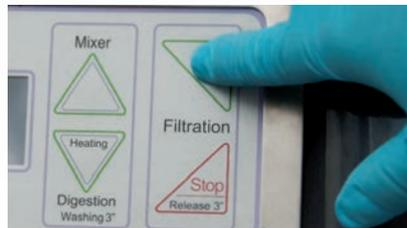
Stop the pump by pressing stop for 1/2 second.
