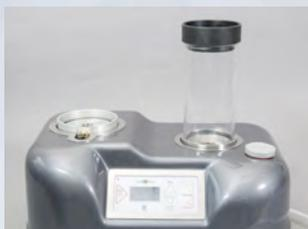
When the digestion is completed, put the resulting product into the filtering container and start the filtering program pressing "Start" button, which will launch the total unload of the digested sample.
