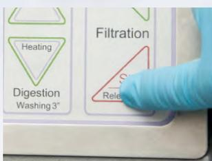
Press "Stop" if you need to interrupt filtering process.
